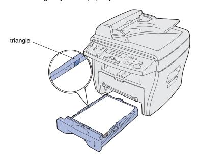
5 Squeezing the paper guides as shown, move the guides until they lightly touch the side of the stack of paper.
